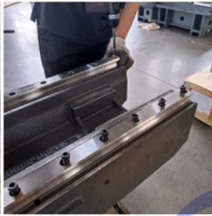
Line guide rail installation, using code meter accuracy test.
