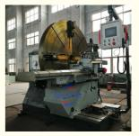
C6030 Flange Lathe Horizontal Facing Lathe Machines for Turning Aluminum Wheel
