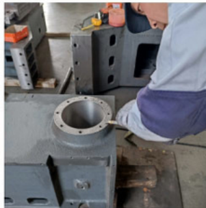
Each contact surface of the workpiece is manually scraped to ensure the precision of the machine.
