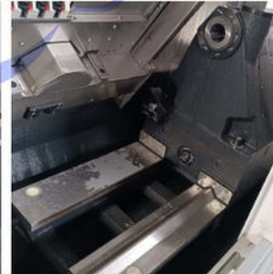
A convex and a flat tailstock design
