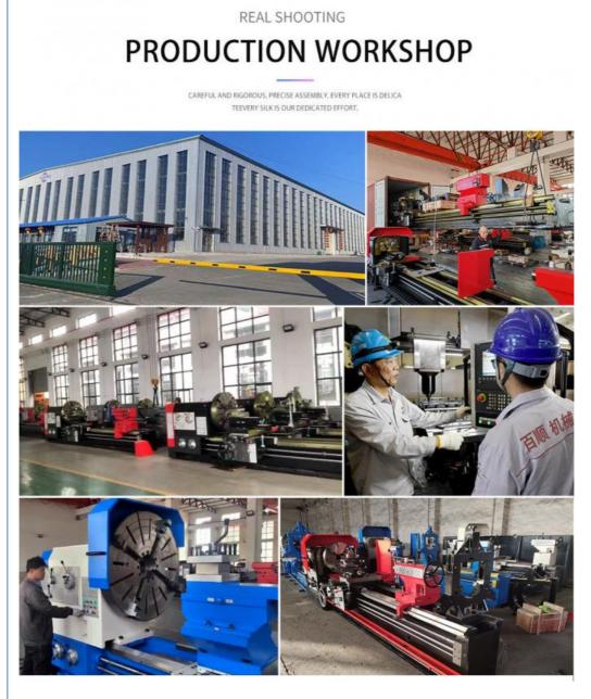
Our metal lathes are mainly suitable for cutting the workpiece inside and outside of shafts, discs and cylindrical, taper surfaces, arc surfaces and other rotating parts, machinable various commonly used metric, inch, module and diametral pitch thread, and boring holes, teaming holes and machining noncircular curved surfaces ect.
