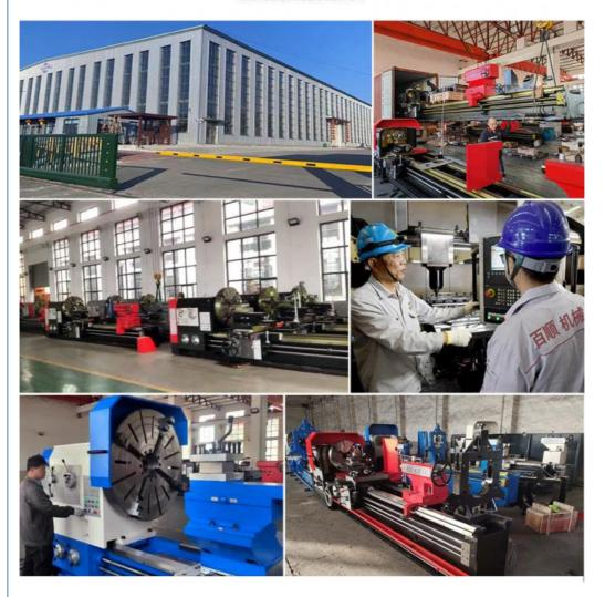
Our metal lathes are mainly suitable for cutting the workpiece inside and outside of shafts, discs and cylindrical, taper surfaces, arc surfaces and other rotating parts, machinable various commonly used metric, inch, module and diametral pitch thread, and boring holes, teaming holes and machining noncircular curved surfaces ect.
