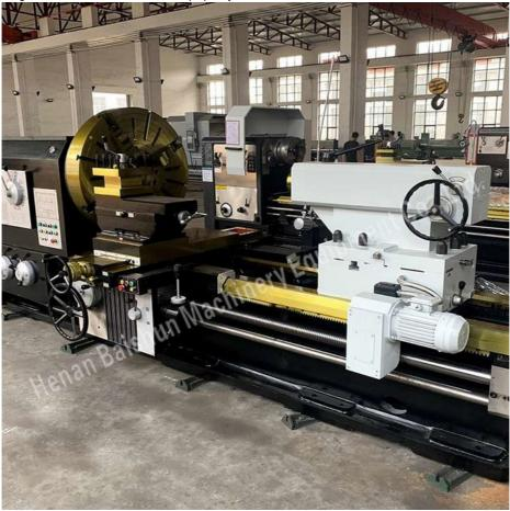
CW61125B Series Lathe Machine( 6 tons load capacity): Swing over bed: 1250mm; Swing over cross slide: 860mm; Processing length: it's up to customer's requirements; Bed width: 755mm; Load capacity: 6 tons; Spindle bore: 130mm; Main motor power: 22kw.
