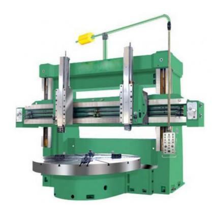
The heavy duty vertical lathe machine is one of my company's own developed vertical lathes, belonging to large universal metal-cutting processing equipment. The product uses advanced CAD computer-aided design techniques, in accordance with national, industry-related design and manufacture of acceptance standards.
