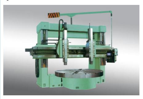
Vertical lathe is suitable for the industries of mechanical processing, can be used for inside and outside the cylinder, cone surface and face, cutting, cutting, etc.
