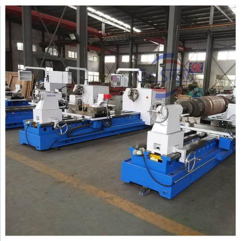
CNC Roller Lathe Machine for processing rolling mill mainly used for semi-finish turning and finish turning processing of cast iron, steel and nonferrous metal roll. Cutters made of high-speed steel. This lathe can be used for turning and processing roll excircle, end faces, various complex pass profiles and curved surfaces, or for the processing of shaft parts made of materials such as cast iron, steel and nonferrous metal.
